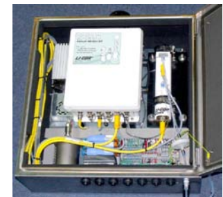
Top-Box with independent Air-CO 2 Analyzer LI-7200, GPS and interfaces to meteo. Sensors. Simple data interface to the OceanPack system.
